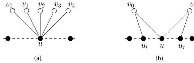
**Fig. 2.** (a) A star of mobile vertices of degree one attached to the same fixed vertex  $u$ . (b) The extremal vertices  $v_0$  and  $v_h = v_4$  can be made vertices of degree two by connecting them to two dummy fixed vertices  $u_l$  and  $u_r$  close to  $u$ . The other mobile vertices attached to  $u$  are temporarily removed and trivially reinserted in the drawing at the end of the drawing algorithm.
