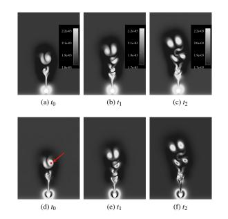
Figure 10: Temporal evolution of the HKS for the heated cylinder with  $A_1 = 0$ . Top row: Mean HKS with scale range [0, 0.5]. Bottom Row: Point Similarity with respect to the red selected point in (d).
