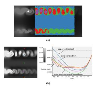
Figure 8: (a) Flow over double cylinders using k-means clustering with k = 4. (b) Five points with their HKS curves.
