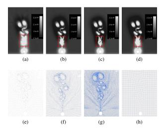
Figure 12: A comparison where both number and spatial distribution of pathlines vary. Top: Mean HKS of the  $A_0$  heated cylinder dataset with different spatial distribution of pathlines. Bottom: Starting positions of the pathlines in the above sample. Number of pathlines: (a) 16572 (b) 74205 (c) 175518 (d) 123493.
