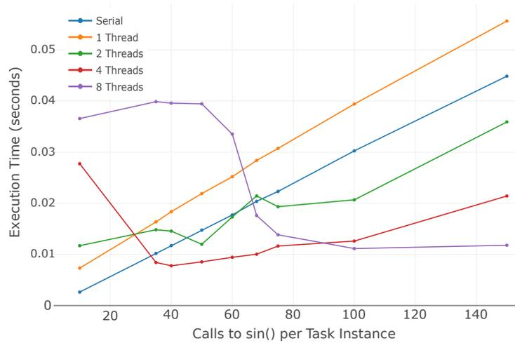
(b) Execution time scaling with number of threads and amount of discovered parallel work. As the work per iteration crosses the equivalent of 35 calls to sin(), our method run on four threads executes faster than the original C serial code.
